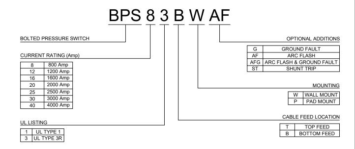
This chart represents the most common models, equipped with 3 poles and 4 wires. There are many other models available, please contact us for configurations not shown here.
