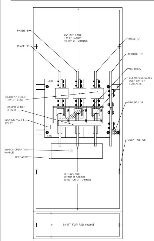
Dimensions shown are for 800-3000 Amps (4000 Amp Dimensions shown in Parenthesis)
